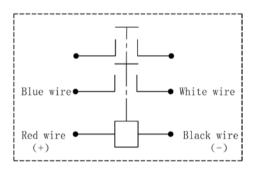
Note: The coil has polarity, The load and Aux. have no polarity
